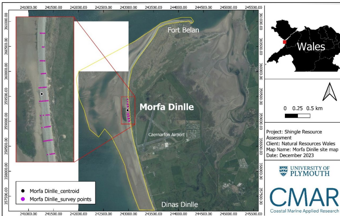
Figure 4: Morfa Dinlle site map. Yellow polygon indicates the extent of the composite gravel and sand spit system. Survey area is highlighted by zoom box, with purple points indicating each of the 50 digital sediment samples collected. No RTK-GPS profiles were available from the WCMC for this study site. Aerial images © Bluesky International Limited and Getmapping 2024
