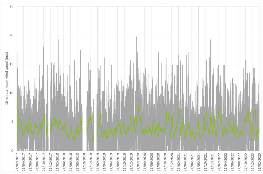
Figure 8: A timeseries of 10-minute mean wind speed, displayed as a raw data (grey line) and a 14 day rolling average (green line).
