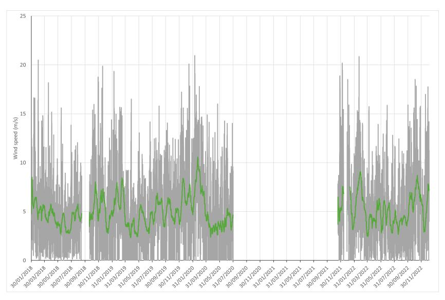
Figure 3: A timeseries of 10-minute mean wind speed for Newborough; raw data is show as grey line and 14 day rolling average shown as a green line.
