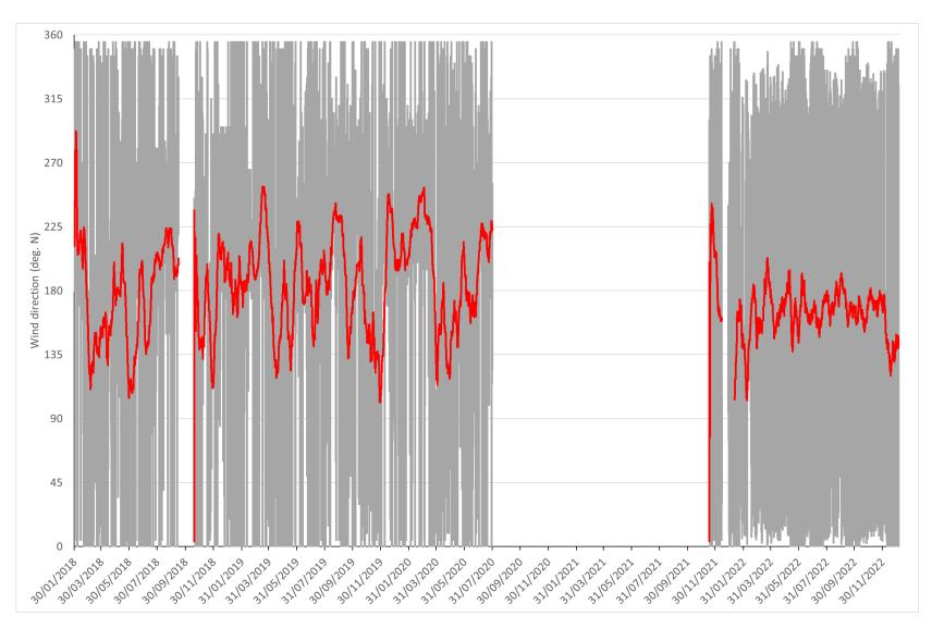
Figure 4: A timeseries of wind direction at Newborough, the data is displayed as raw data (grey line) and a rolling average over 14 days (red line).
