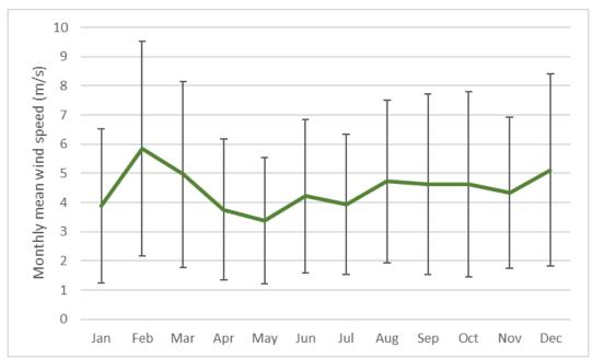
Figure 34: Monthly average 10-minute-mean wind speeds (green line) and monthly standard deviation in 10-minute-mean wind speeds (vertical bars) for Merthyr Mawr.
