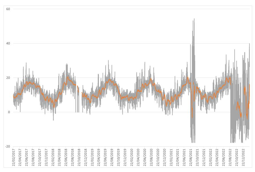
Figure 20: Temperature at Whiteford, displayed as raw data (grey line) and 14 day rolling average (orange line). The sensor malfunctioned after 08/2021.
