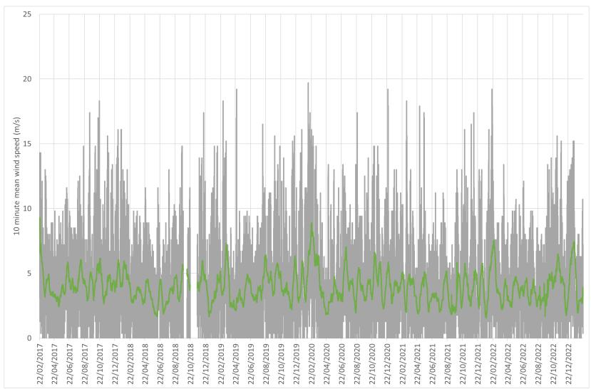
Figure 18: A timeseries of mean 10-minute wind speed at Whiteford, displayed as raw data (grey line) and 14 day rolling average (green line).
