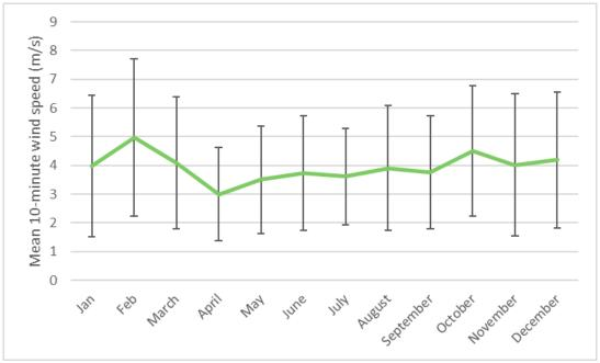
Figure 24: Monthly averages of 10 minute mean wind speed (green line) and standard deviation (vertical bars) at Whiteford.
