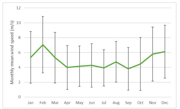
Figure 7: Monthly averages (green line) and standard deviations (vertical bars) in wind speed (m/s) for Newborough. Averages are calculated over all years where data is available.
