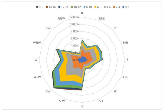
Figure 5: A wind rose (m/s) for the Newborough data from all years and seasons. Wind speed is indicated by colour shading, direction by the compass points and percentage proportion of occurence on the radial axis.
