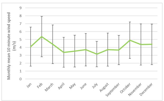
Figure 14: Monthly average (green line) and standard deviation (vertical bars) of 10-minute mean wind speeds at Morfa Harlech.
